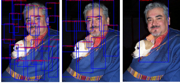
Figure 5. Examples of size bias in detection windows where detection windows are limited to the highest 10, 5, and 3 levels of the pyramid
